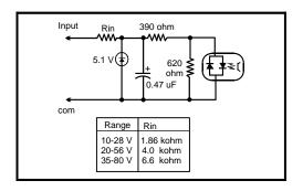
Typical Termination Panel Input Circuit
