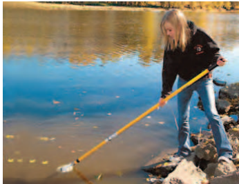
The swing sampler allows for easy sample collection from different angles. Pole extends up to 12 ft.
