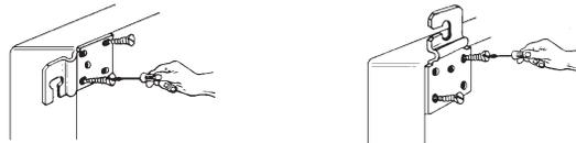
Figure 5. Plastic Housing - Mounting Brackets Installation
