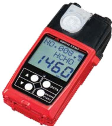
The FP-31 is a highly specific gas detector utilizing a proprietary colorimetric paper tablet to detect Formaldehyde. The instrument has a digital readout of the gas concentration on an LCD display. Readings are of average formaldehyde exposure over a selectable 15 minute or 30 minute period. This instrument does not respond to typical interference gases such as acetaldehyde, acetone, alcohols, ammonia, benzene, carbon monoxide, toluene or xylene.
