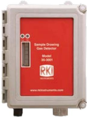
The 35-3001 series is a compact sample draw detector assembly with a built-in pump that accepts a 24VDC input. This unit features a NEMA 4X enclosure making it dust, water and corrosion resistant. It also features a flowmeter with adjustable flow and a low flow alarm which warns of any obstructions or restrictions in the flow system. The 35-3001 is also available in some dual sensor configurations.
