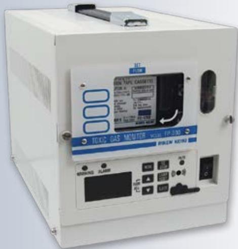
RKI's paper tape monitors utilize highly sensitive colorimetric tapes to achieve interference free detection at low PPB and PPM levels of a wide variety of gases. Each model is equipped with easily replaceable tapes that are specific to the gas being monitored. Each model has a digital display showing the type of gas and concentration in either PPM or PPB, and also displays remaining tape time as well as an end of tape alarm.
